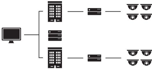
The distributed architecture leverages a separate management server and one or more recording servers for more scalable applications. Each recording server operates autonomously for maximum reliability across multiple locations.
